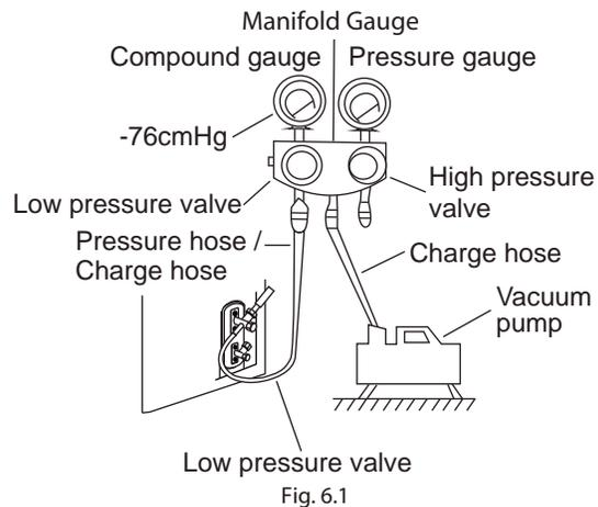
1. Connect the charge hose of the manifold gauge to service port on the outdoor unit's low pressure valve.
